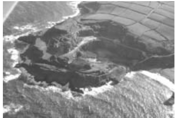
Figure 3: West of England Quarry, Porthoustock. This Gabbro quarry is typical of aggregates quarries in having few waste dumps and the interior is relatively formless. Few structural remains survive here except parts of the jetties. Prograded beach at Porthoustock shows on the right. (c. Historic Environment Service, Cornwall County Council)
